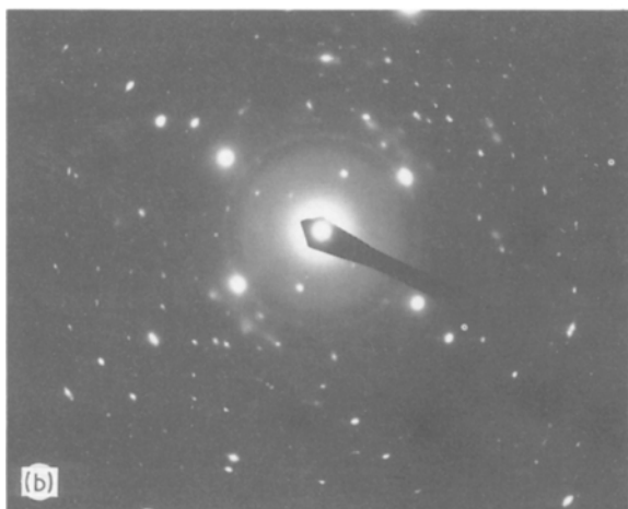
Figure 4 (a) Bright-field electron micrograph of \text{Fe}_{78}\text{Si}_{10}\text{B}_{12} annealed at 773 K for 1 h showing a typical spherical eutectic cell containing \alpha -iron and \text{Fe}_3\text{B} . (b), (c) Electron diffraction pattern and schematic drawing taken from eutectic cell in (a). (○) Reflections from the \alpha -iron phase, (●) reflections from the boride phase.
